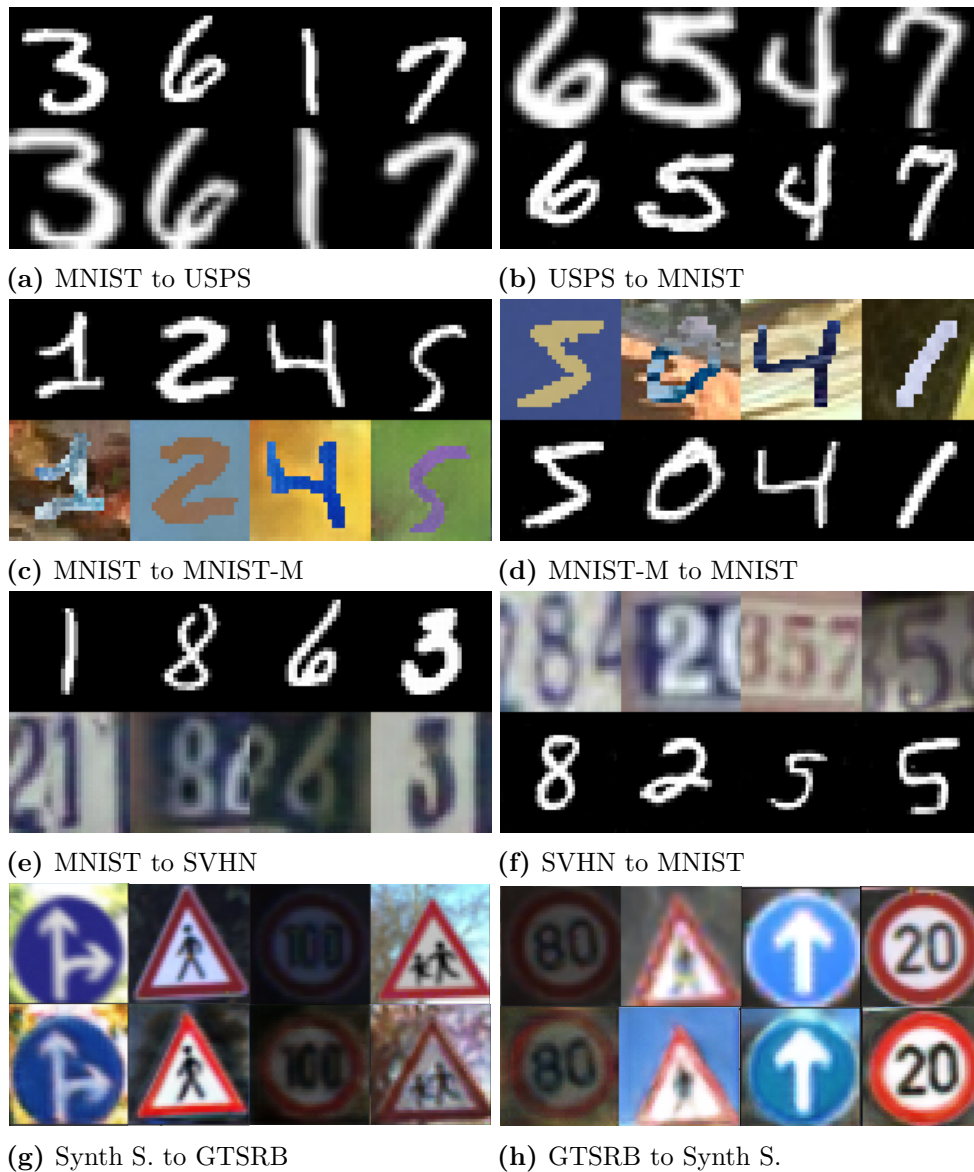
Figure 4.3. Examples of generated digits: we show the image transformation from the original domain to the paired one as indicated under every sub-figure. For each of the (a)-(h) cases, the original/generated images are in the top/bottom row.
